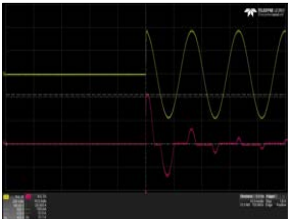
Figure 23: LPS365-M Inrush Current Vin = 264Vac Load: Io = 0A, Turn on at 90 deg Ch 1: V IN Ch 2: I IN
