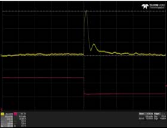
Figure 17: LPS364-M Transient Response – Vo Deviation Vin = 90Vac Load: Io = 100% to 50%, 1A/us slew rate Ch 1: Vo Ch 2: Io
