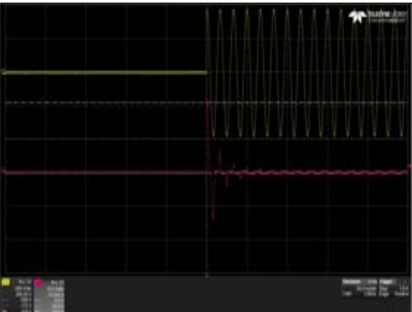
Figure 33: LPS366-M Inrush Current Vin = 264Vac Load: Io = 0A, Turn on at 90 deg Ch 1: V IN Ch 2: I IN
