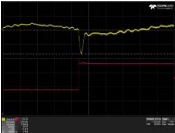
Figure 48: LPS368-M Transient Response – Vo Deviation Vin = 90Vac Load: Io = 50% to 100%, 1A/us slew rate Ch 1: Vo Ch 2: Io
