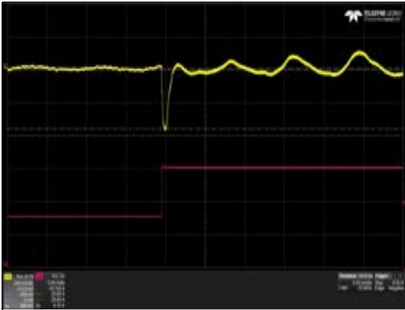
Figure 28: LPS365-M Transient Response – Vo Deviation Vin = 90Vac Load: Io = 50% to 100%, 1A/us slew rate Ch 1: Vo Ch 2: Io
