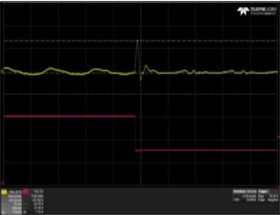
Figure 27: LPS365-M Transient Response – Vo Deviation Vin = 90Vac Load: Io = 100% to 50%, 1A/us slew rate Ch 1: Vo Ch 2: Io
