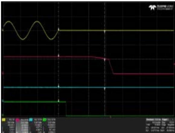
Figure 22: LPS365-M Hold-up Time (time to decay) Vin = 90Vac Load: Io = 15A, I SB = 1A Ch 1: V IN Ch 2: V O Ch 3: V SB Ch 4: Power Fail
