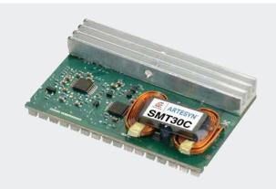
Advanced Energy's Artesyn SMT30C series surface mount 30 amp non-isolated DC-DC converter is designed for cost- and space-sensitive applications. It accepts a 10.2 to 13.8 Vdc input and provides an output that is adjustable from 0.9 to 5.0 Vdc to accommodate a wide variety of silicon power needs. Rated at 150 watts, the converter has a typical efficiency of 91%. Standard features include remote sense, remote On/Off and remote 'power good' indication.
