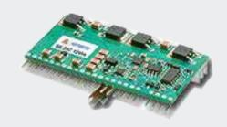
Advanced Energy's Artesyn SIL25C series 25 amp high density non-isolated DC-DC converter is designed for cost- and space-sensitive applications. It accepts a 10.2 to 13.8 Vdc input and provides a negative 5.05 Vdc output. Rated at 125 watts, the converter has a typical efficiency of 90%. Standard features include remote sense, remote On/Off and remote 'power good' indication.
