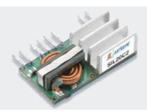
Advanced Energy's Artesyn SMT20C2 series surface mount 20 amp non-isolated DC-DC converter is designed for cost- and space-sensitive applications. It accepts a wide range 4.5 to 13.8 Vdc input and provides an output that is adjustable from 0.59 to 5.1 Vdc to accommodate a wide variety of silicon power needs. Rated at 100 watts, the converter has a typical efficiency of 93%. Standard features include remote sense, remote On/Off and remote 'power good' indication.
