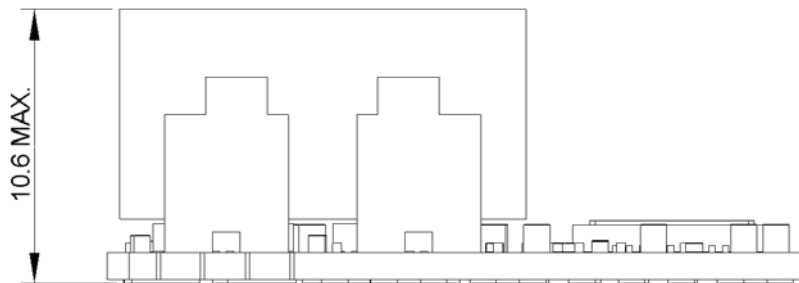
Side view of standard profile solder bump termination type (LGA50D-01DADJSBJ)
