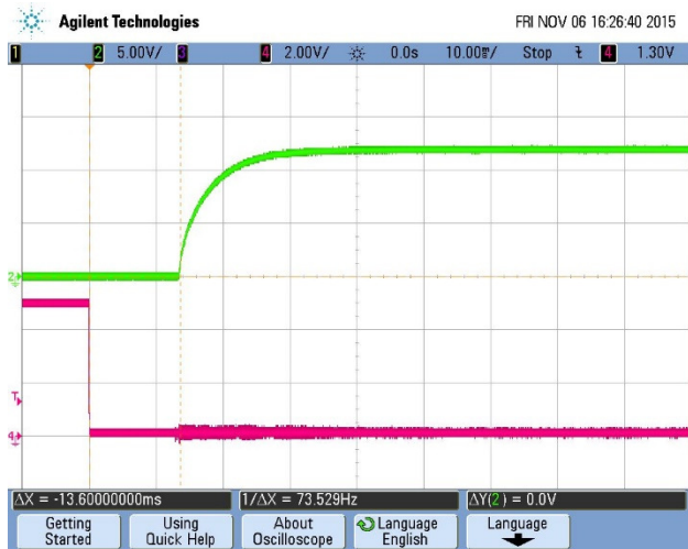
Figure 15: Turn-on transient at zero load current (10 mS/div, Top Trace: Vout, 5V/div; Bottom Trace: ON/OFF, 2V/div)
