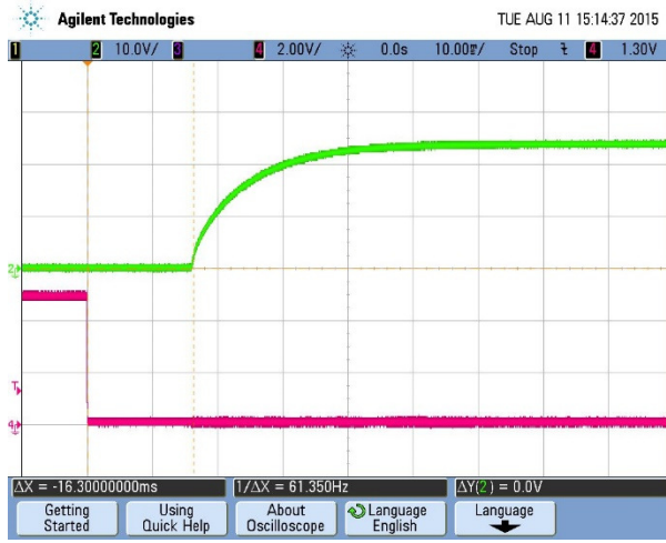
Figure 27: Turn-on transient at zero load current (10 mS/div, Top Trace: Vout, 10V/div; Bottom Trace: ON/OFF, 2V/div)
