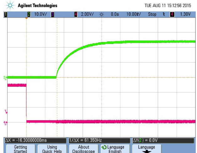
Figure 28: Turn-on transient at full load current (10 mS/div, Top Trace: Vout, 10V/div; Bottom Trace: ON/OFF, 2V/div)
