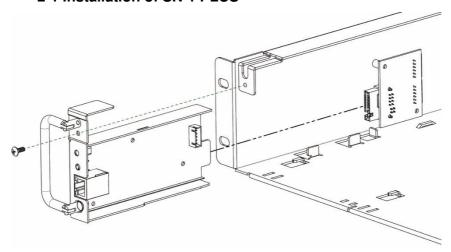
Step 1: Hold the button on the panel and slot in the SN-1 PLUS card for 1 second
